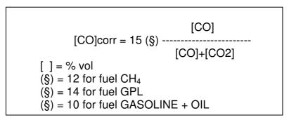
when the sum of [CO] and [CO2] is less than 15 for gasoline fuel, 14 for GPL fuel, 12 for Methane fuel, 10 for GASOLINE + OIL fuel; in the other cases the test result is the one showed by the instrument.
