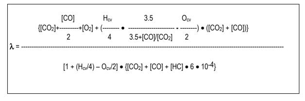
$\begin{array}{ll} H_{CV} = & 1.73 & \text{GASOLINE fuel} \\ & 2.525 & \text{GPL fuel} \\ & 4 & \text{METHANE fuel} \\ O_{cv} = & 0,02 \\ [CO], & [CO_2] & e & [O_2] = \% \text{ in vol.} \\ [HC] = & \text{ppm in vol.} \end{array}$
