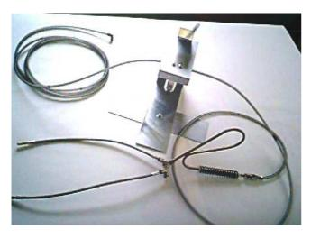
In alternative, flexible terminals can be used, these are more protected against detritus because suction holes are lateral. To perform a measure with multiple exhaust pipes, connect to the brass pipe 3 "Y" unions, with the needed flexible terminals, close the holes not used with the dedicated caps.
