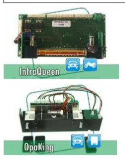
In the field of emission test, Assemblad has long since been using its own proprietary technology: it's the INFRA QUEEN oiml class 00 4/5-gas bench and the OPA KING ISO 11614 and SAE J1677 partial flow smoke bench that equip all Assemblad emission testers for Workshops and Inspection Centres. In an industry where changes on emission tests are closely on the way, a true emission tester manufacturer gives the guarantee that the products will keep up for the new coming inspection procedures.
