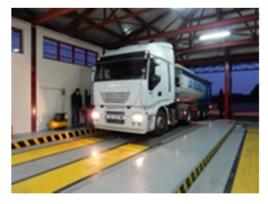
According to a study carried out by AICA, the Italian Association of garage equipment manufacturers, under the mandate of the Italian Ministry of Infrastructure and Transport, plate brake testers and roller brake testers are both suitable for PTI as the testing results from both testing methods correlate. Therefore, a plate brake tester, which is approved by several national Authorities for statutory tests, is perfectly fit for PTI as well as for pretest and repair assessment.
